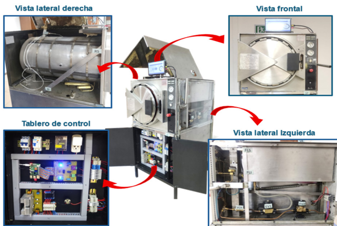
Figure 1. Shows the final teaching equipment, the result of the modernization process. Pelton et al. autoclave modified as a teaching tool, showing the interior of the sterilization chamber and components of the new control system (sensors, wiring, and actuators)
