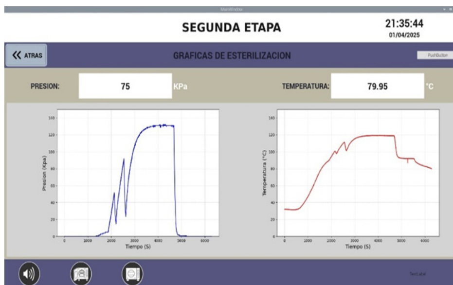
Figure 6. Final graph of the sterilization cycle
