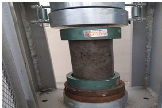
Figure 2. Alignment of the sample axis with the center of thrust of the press
