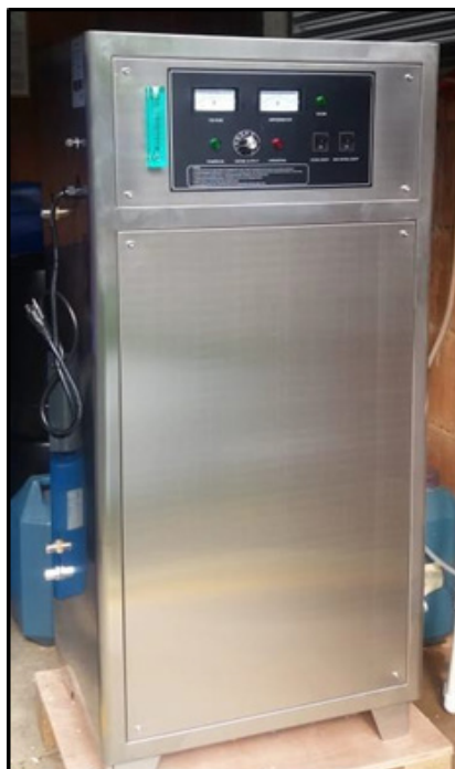
Figure 16. Photograph of the ozone generation system WTC S.A.S
